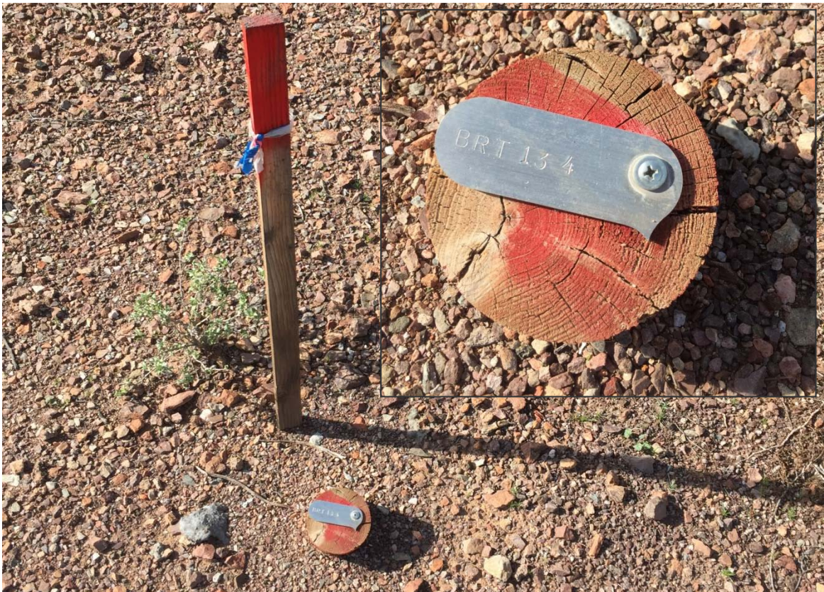
Figure 6-3: Drill hole monument
